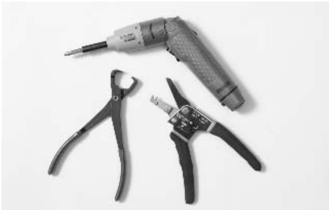
Figure 1. Face mask removal tools, counterclockwise from the top: cordless screwdriver, Trainer's Angel, and the FM Extractor.
