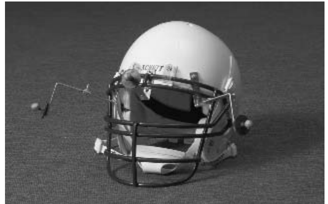
Figure 3. Helmet marker setup.
